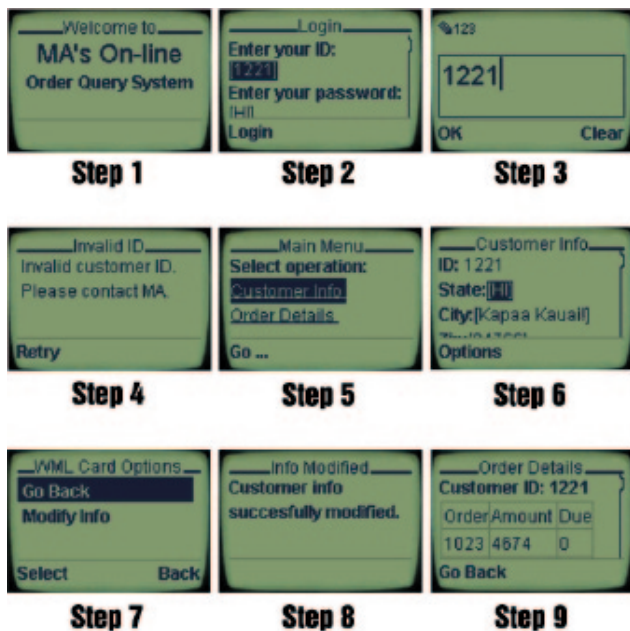
Figure 7: Screens of the Nokia 6110 simulator. The steps indicate the order of appearance in MAOOQS.
